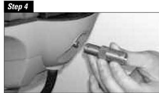
Step 4 First hand-screw the Quick Clear adapter onto the valve.
