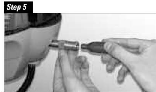
Step 5 While holding the adapter in place, screw the Quick Clear cartridge into Quick Clear adapter.
