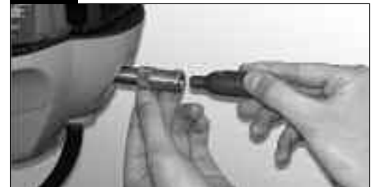
While holding the adapter in place, screw the Quick Clear cartridge into Quick Clear adapter.
